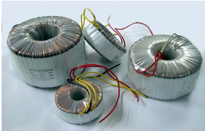
Figure 8. Common used pulse transformers with closed toroidal magnetic cores
